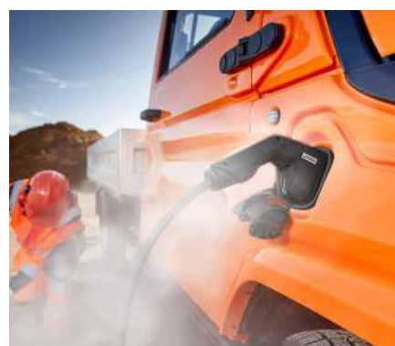
With charging connector plugged in: IP44B/IP44D
