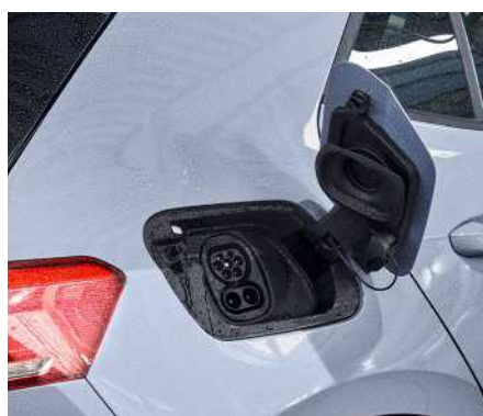
With vehicle charging inlet uncovered: IP6K6K/IP6K9K
